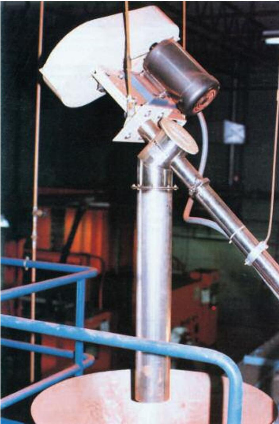
**The spiral conveyor's drive motor and discharge are suspended above the ferrite manufacturer's rotary calciner.**
